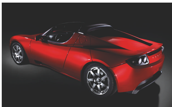
The Tesla Roadster EV relies on a battery pack employing about 6800 lithium-ion cells, enabling it to go from 0 to 60 mpg in 4 seconds, with a range of more than 200 miles.
